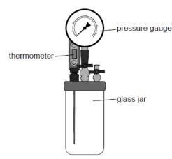
The apparatus is cooled in a freezer and then placed in a water bath so that the temperature of the gas increases slowly. The pressure and temperature of the gas are recorded.
