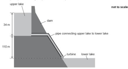
The water leaving the upper lake descends a vertical distance of 110 m and turns the turbine of a generator before exiting into the lower lake.
