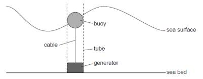
The motion of the buoy can be assumed to be simple harmonic.
