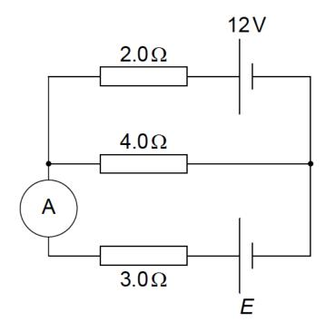
The top cell has electromotive force (emf) 12V. The emf of the lower cell is unknown. The ideal ammeter reads zero current.
