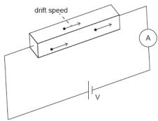
The following data are available for the conductor: density of free electrons =  $8.5 \times 10^{22} \text{ cm}^{-3}$ resistivity  $\rho = 1.7 \times 10^{-8} \Omega \text{m}$ dimensions w × h × l = 0.020 cm × 0.020 cm × 10 cm. The ammeter reading is 2.0 A.
