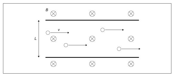
(i) Show that the potential difference V that is established across the conductor is given by V=vBL.
