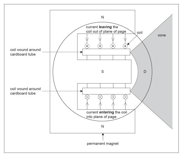
The coil consists of 150 turns, each of average diameter 2.5 cm. The magnetic field of the permanent magnet has strength 0.40 mT. The peak current in the coil is 0.45 mA.
