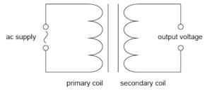
The transformer has 100 turns in the primary coil and 1200 turns in the secondary coil. The peak value of the voltage of the ac supply is 220 V. Determine the root mean square (rms) value of the output voltage.
