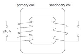
The number of turns in the primary coil is 1800 and that in the secondary coil is 90.
