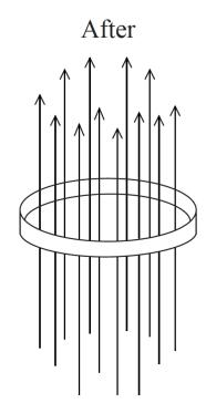
field caused by (induced) current must be downwards; to oppose the change that produced it; hence the current must be clockwise;
