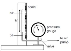
The pump forces oil to move up the tube decreasing the volume of the trapped air.
