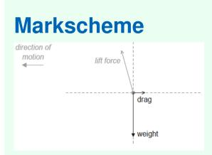
drag correctly labelled and in correct direction
