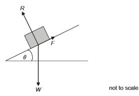
What is the maximum coefficient of static friction between the block and the plane?
