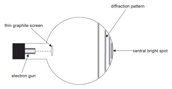
A pattern forms when diffracted electrons are incident on a fluorescent layer at the end of the tube.
